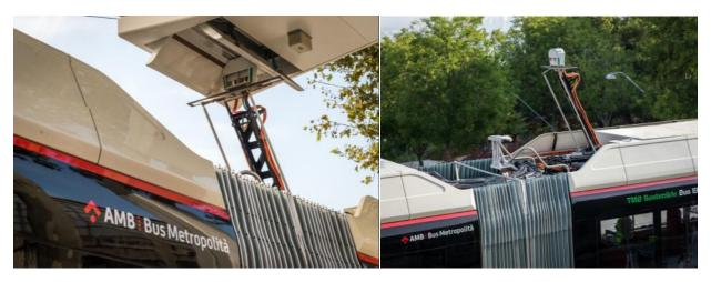
The pantograph connects to the top part of the rapid charge station On the right, a view of the on-roof retractable arm of the Solaris Urbino 18E
